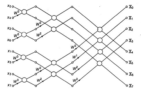
Where  $W^j$  is one of the frequencies in the DFT calculation (= $2\pi j/N$ ). This **signal flow graph** is the basis of the ComplexFFT() implementation. To operate the graph, the input signal is shuffled into the spectrum array in an order known as **bit-reversed addressing**. Then each column of butterfly operations is performed, so that the signal 'moves' left-to-right through the graph, turning into the DFT spectrum.
